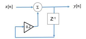
(iii) Impulse response is the response of this filter an unit impulse, i.e. x[n] = [1,0,0,...]Therefore, y[n] = [0, 0.2, 0.04, 0.008, 0.0016, 0.00032, ...].
