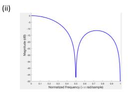
(ii) 1 Hz is very small compared with the sampling rate of 10 kHz therefore the filter will simply pass the signal through (lowpass). 4.5 kHz is nearly half the sampling frequency; therefore, this filter will attenuate significantly the signal at this frequency.
